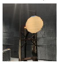
G Systems' Radome Transmissivity Test Software is the final component to the fully automated system. It includes several operating modes, the primary of which is a wizard-style step-by-step process. The wizard interface walks an operator through the automatic calibration and prompts for loading and testing of a radome. The software also includes a manual operation mode, allowing the user to test a radome by moving it to a particular set of angles and taking a singular
