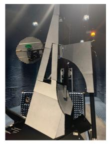
standard. This includes measuring from -80 degrees to +80 degrees around the radome's azimuthal axis and from -20 degrees to +20 degrees on the elevation axis.
