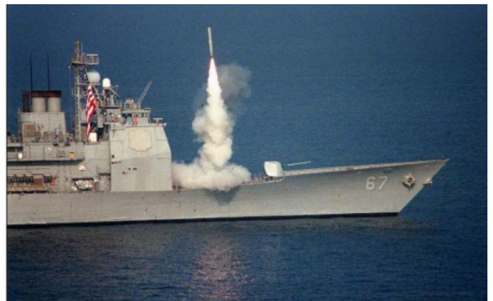
Figure 1. A Tomahawk missile released from the MK 41 VLS (photo courtesy of U.S. Navy)
