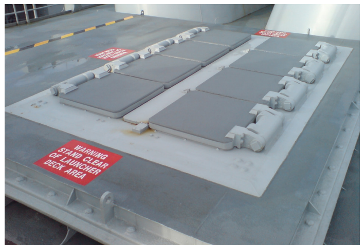
Figure 4. Each VLS module contains eight missile-loaded canisters
