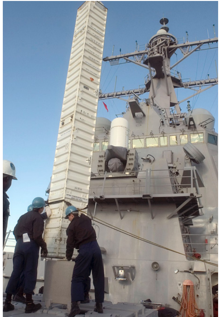
Figure 3. A loaded canister is lowered into one VLS module
