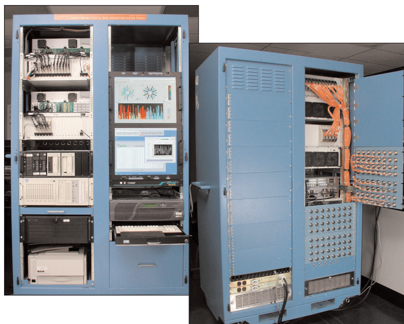
Figure 3 – Integrated PDDAS system supporting 128 channels
