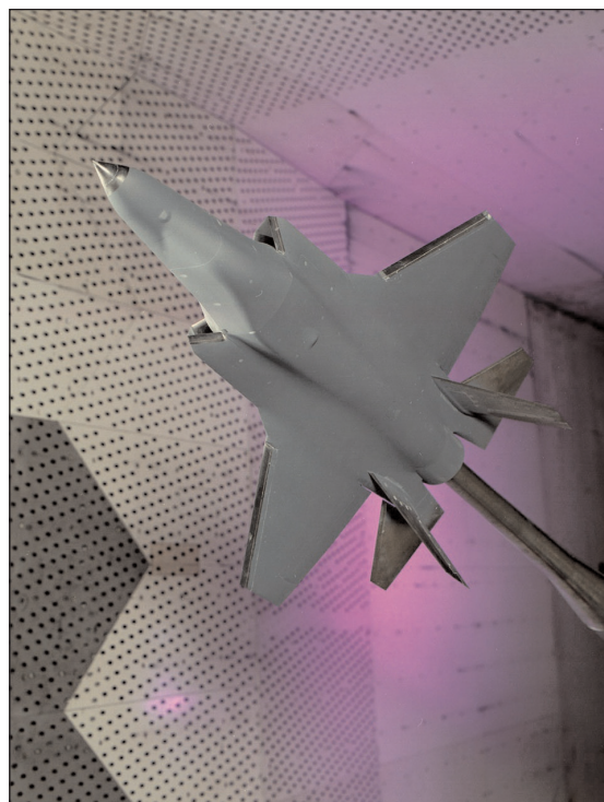
Figure 4 – F-35 scale model in transonic wind tunnel
